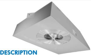
The JISU Series of JetVent Fans are available in 50 and 100N thrust capacities. This range is suitable for ambient and also high temperature applications as required in fire/smoke control applications. All models feature a low profile housing that is suitable for car parks with low ceiling heights. These units may be used in conjunction with Variable Speed Drives (VSD) for efficient speed control.
