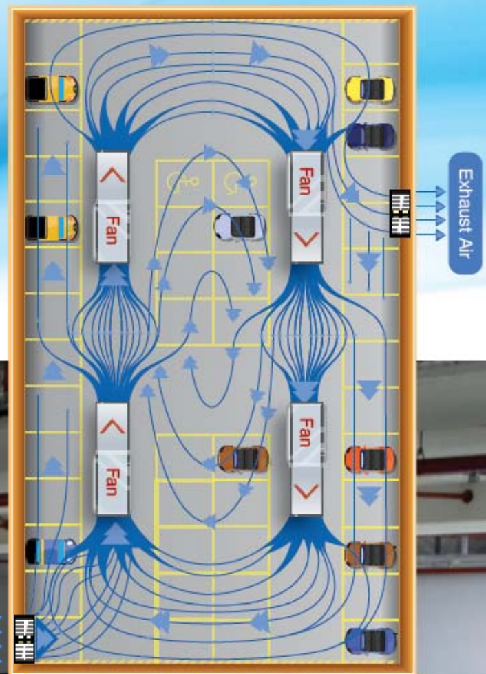
Figure 5. Circular mixing system
