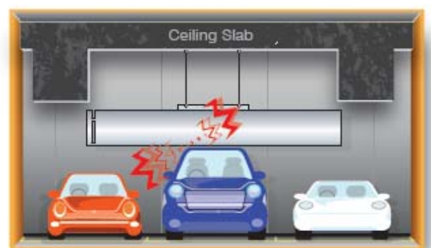
Figure 8(b). Insufficient clearance
