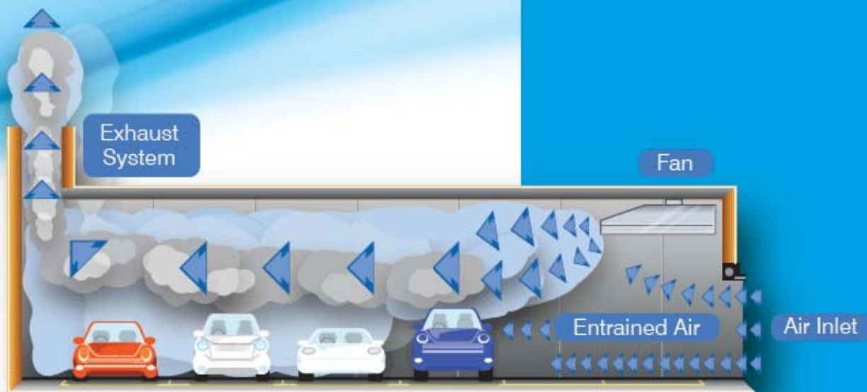
Figure 2. Workings of a JetVent or Impulse fan
