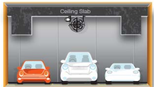
Figure 8(a). Sufficient clearance
